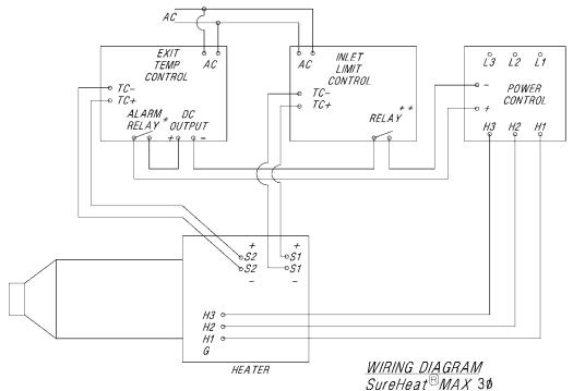
\* EXIT TEMP ALARM RELAY TO OPEN AT 1405°F. \*\* INLET LIMIT RELAY TO OPEN AT 250°F. OTHER SETTINGS MAY DAMAGE HEATER AND VOID WARRANTY.
