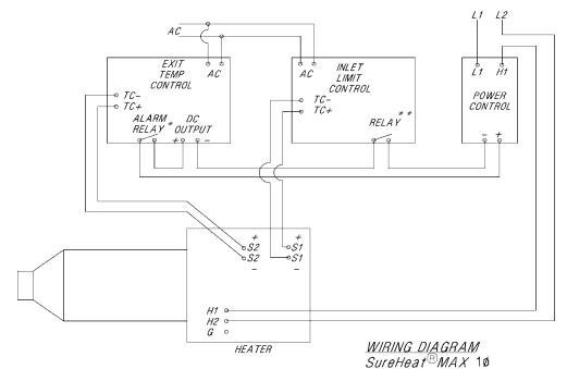
\* EXIT TEMP ALARM RELAY TO OPEN AT 1405°F. \*\* INLET LIMIT RELAY TO OPEN AT 250°F. OTHER SETTINGS MAY DAMAGE HEATER AND VOID WARRANTY.
