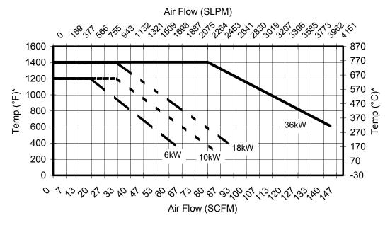
\* Temp as measured by internal "K" thermocouple.
