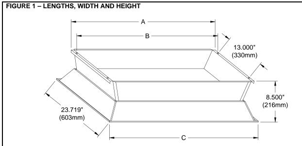
Note: Four (4) mounting holes .375" (9.5mm) diameter for balanced suspension are located by dimensions B x 13.000" (330mm).
