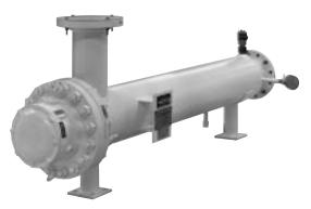
**Military Lube Oil Heater:** These lubrication oil circulation heaters are used on U.S. Naval ships. This design exemplifies INDEECO's ability to manufacture special equipment in compliance with detailed specifications such as MIL-SPEC requirements which can include performance, shock and vibration tests.
