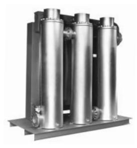
**Fuel Oil Heater System:** A 209 KW fuel oil heater which includes a built-on Vernier control system. The low watt density requirements resulted in a 20 foot long vessel design with immersion heaters inserted at each end.
