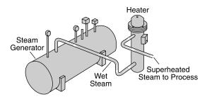
Fuel oil heating where the circulation heater raises the temperature of fuel oil to reduce its viscosity, facilitating its flow into the burner.
