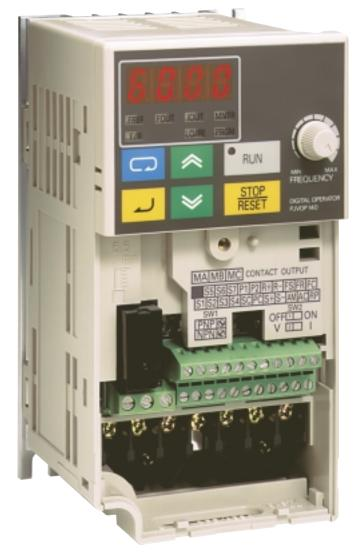
Wiring the 3G3MV is simple with easy to use screw terminals that accept 0 -10 V, 4-20 mA or 0 - 20 mA analog signals or pulse train inputs between 0.1 kHz and 33 kHz (scalable). It also offers analog and digital outputs for direct monitoring and control. The multi-function inputs can be set to either PNP or NPN providing flexibility in input signals.
