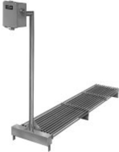
**Sludge Leg Spacers** - To prevent burnouts from spot overheating and to keep elements out of sludge that normally collects in the bottom of the tank. Standard legs are 1-1/2" high; lengths up to 4" are available at no extra charge.
